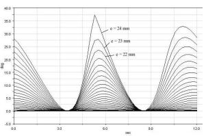
Fig. 10. Relative motion in joint I, J
