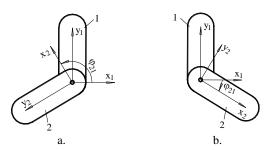
Fig. 5. Joint relative rotation angle measurement
